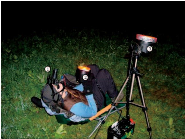
Figure 1. Method for observing and recording activity of bats and birds at wind-energy projects using night-vision goggles and 2 supplementary light sources equipped with infrared filters (B. A. Cooper, Alaska Biological Research, Inc., unpublished data).
