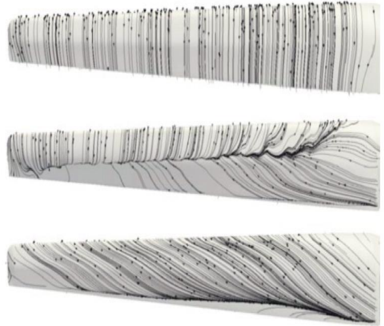
Figure a. Surface streamlines for incoming flow of 5, 10, 21 m/s
